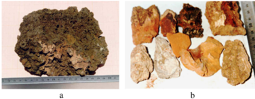
Fig. 6. Slag from the flue gas duct (a), and slag and fouling fragments from various boiler sections (b).
